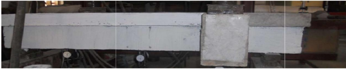
T-beam with a 350mm flange width and no GFRP, control beam (T3C)
