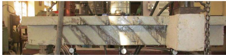
T-shaped beam reinforced using 45° inclination-wrapped GFRP strips
