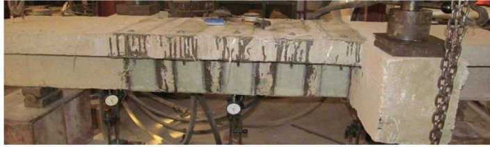
T-shaped beam reinforced with U-Wrap GFRP and flange anchoring.
