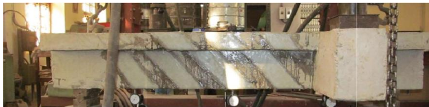
T-shaped beams reinforced using 45° inclination-wrapped GFRP strips
