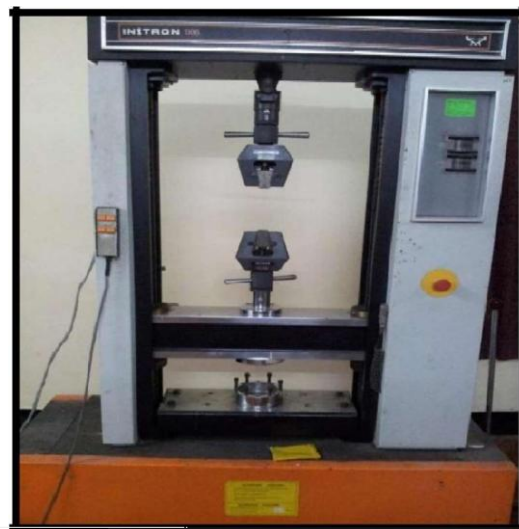
INSTRON universal testing experimental configuration 600 kN capacity machine
