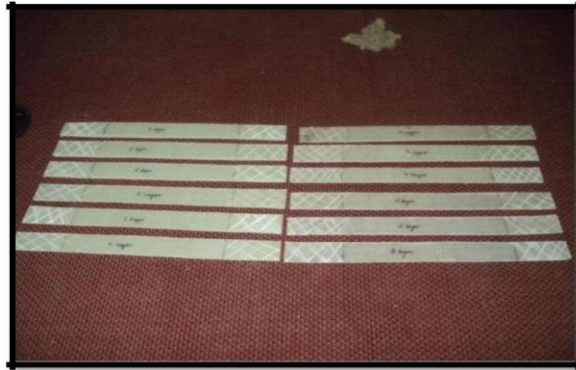
Test specimens for woven glass/epoxy composite tensile tests
