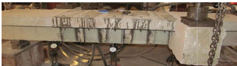
T-shaped beam reinforced with flange anchoring and GFRP of U- Wrap.
