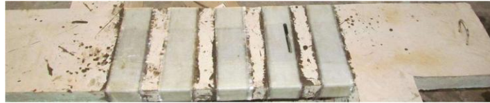
T-shaped beam strengthened using completely wrapped GFRP beams.
